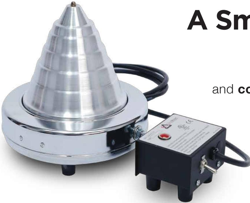
Proper installation is essential to maximize bearing life. Heating a bearing prior to installation expands the inner race cap to allow the bearing to be easily mounted on the shaft. ConeMount Bearing Heaters can help promote bearing longevity which means less equipment downtime and lower maintenance costs.
